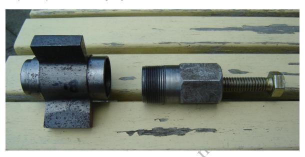
Thread on puller Ø 1 1/4 inch (31, mm) 20 TPI Spannersize 32 mm but any convenient size over 32 mm can obviously be used Centre bolt M10 used, also a free choice but should be big enough but not exceeding the main axle diameter.
